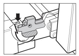
Flip both locking clamps back up to lock them. Turn them as far as they will go into a horizontal position. Make sure that the notches on the locking clamps hook into the slots on the door as illustrated.
